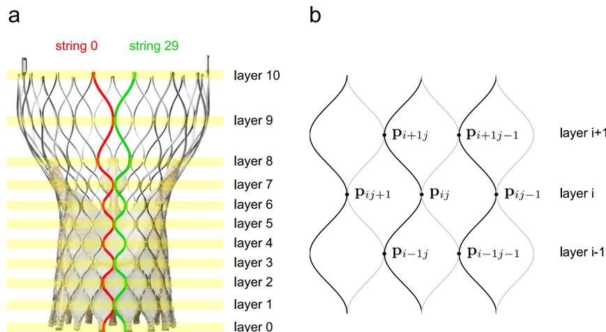
**Fig. 1.** Basic geometric parameter definitions on the CoreValve: The stent can be divided into 11 layers (a). Each layer holds 15 intersection points  $\mathbf{p}_{ij}$ . There are 30 physical strings, which impose a node connectivity pattern for the intersections (b). Layers 0–6 constitute the leaflet area.
