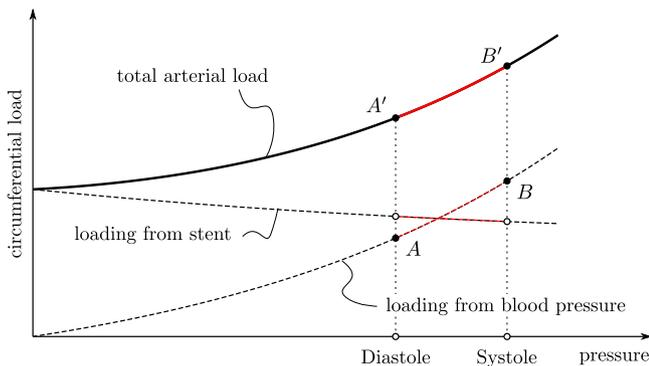
**Fig. 5.** Qualitative depiction of the circumferential loading of the arterial wall as a function of the blood pressure: the loading component of the stent is at a maximum when there is no loading by the blood pressure. Without implant, the loading would be cycling between points A and B. The addition of the stent leads to an elevated cycle between points A' and B'.
