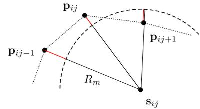
**Fig. 2.** The distortion measures the relative deviation from the average circular radius  $R_m$  at each point  $\mathbf{p}_{ij}$  in a layer.
