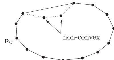
**Fig. 3.** Non-convex points are all points that do not belong to the convex hull of the cross section of the stent.
