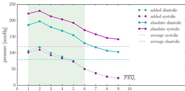
**Fig. 6.** Layer-wise plot of the equivalent pressure: average values for all patients. The dashed straight lines indicate the average human blood pressure in both phases of the heart cycle. The dotted lines correspond to the added pressure in each layer. Both full lines depict the absolute values of pressure-loading in the area, which is the sum of the blood pressure and stent loading. The shaded rectangle indicates the leaflet area.
